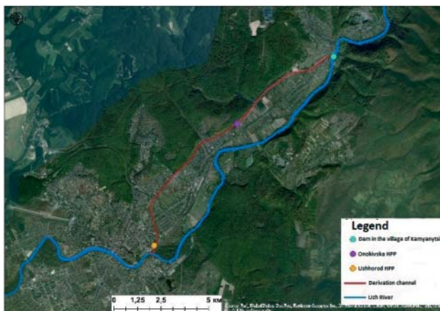
Fig. 2.25. The scheme of regulation of the river Uzh
